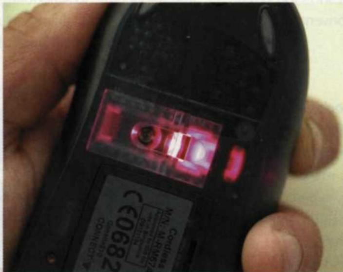
Optical sensor on bottom of cordless optical mouse
